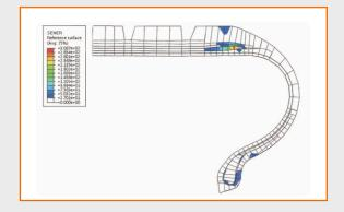
Dual Tread Radius Design distributes stress, enabling longer mileage and helps prevent irregular wear.
