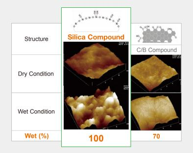
This new hydrophilic material features superior wet grip and braking performance compared to previous carbon compounds.
