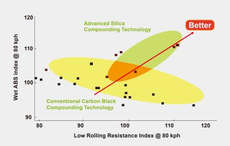
OPTIMO H426 uses an advanced tread silica compound that improves both wet braking and fuel economy.
