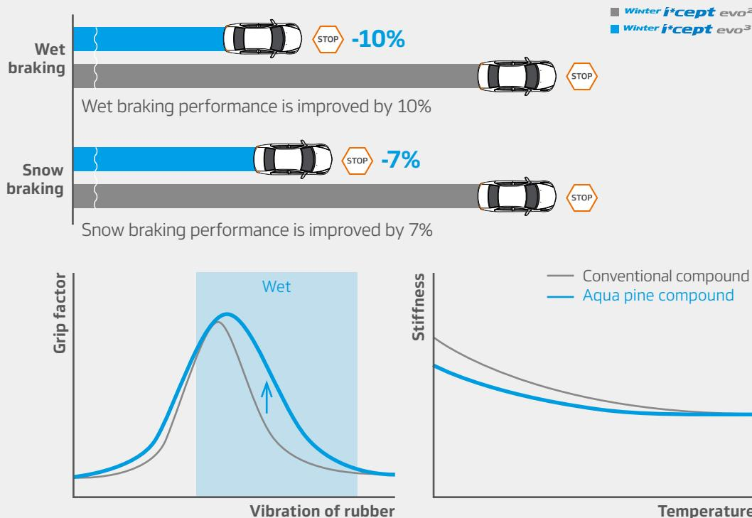
Hankook's advanced mixing technology with high loading silica and traction enhancing additives is used for the tread compound to improve the wet performance.
