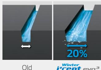
20% wider lateral groove improves water displacing capability compared to winter i\*cept evo<sup>2</sup>.
